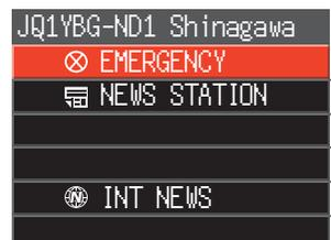
3. Press the **PTT** switch, a beep sounds and a confirmation screen “EMERGENCY Upload?” Appears. When sending emergency information, press and hold the **PTT** switch, after three beeps, the screen display will change to “EMERGENCY UPLOADING” for about 5 seconds, and then the countdown will be started. While pressing the **PTT** switch, speak into MIC.
