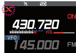
6. When a local node is found, “X” is lit solid, and the node name and city name appear on the bottom part of the screen. Depending on the connection status, the screen will show one of four display patterns.
