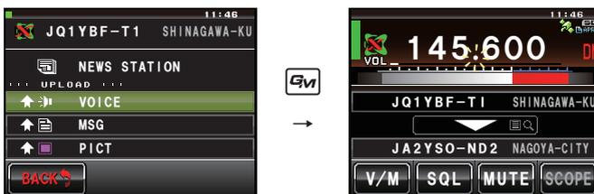
In the connection status display, communication can be switched between Band A or Band B by pressing **[V/M]**.
