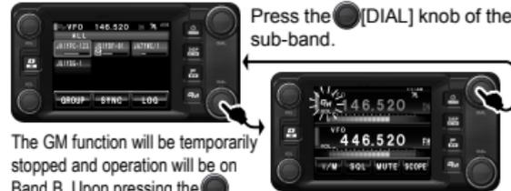
The GM function will be temporarily stopped and operation will be on Band B. Upon pressing the [DIAL] knob of Band A after the sub-band operation, the GM function will resume operation.
