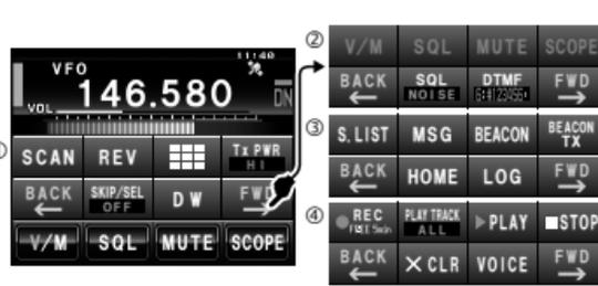
These keys can be substituted by the four operation keys normally displayed at the lower part of the frequency display screen (refer to the operating manual for details).
