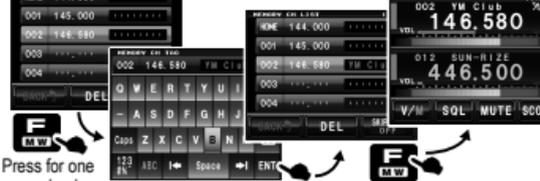
Touch the screen, or turn the [DIAL] knob at the top right of the screen to select the memory channel. After entering the name on the character input screen, press the [F] key for one second or longer, and touch [ENT] to return to the memory list. Press the [F] key again to return to the previous screen.
