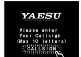
Touch the blinking [CALLSIGN] on the screen to begin inputting the call sign (the display will switch to the character input screen automatically if there are no operations for about 3 seconds).
