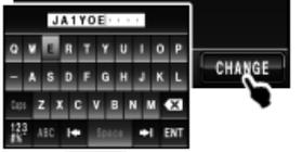
Touch [CHANGE] on the screen and follow the same process as the input procedure to change the call sign or name (moving the cursor to the left end using [←] and [→] and touching [DISP] will return the display to the previous screen without the change being reflected). Press the [DISP] key to return to the frequency screen.
