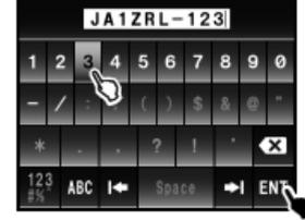
After entering the call sign or name, by touching the characters on the screen, or turning and pressing the [DIAL] knob at the top right of the screen, touch [ENT] on the screen to confirm and enter the call sign.
