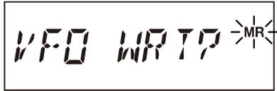
3. Press the [MHz(SETUP)] key, the data will now have been copied to the VFO, although the original memory contents will remain intact on the previously-stored channel.
