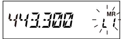
**Note:** While operating in the Memory Storage mode, the keypad of the MH-48A6JA Microphone may be used to enter the memory channel number directly.
