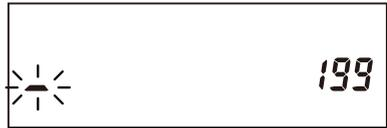
8. When you have programmed a label that is under 8 characters, press the **[MHz(SETUP)]** key to confirm the label.
