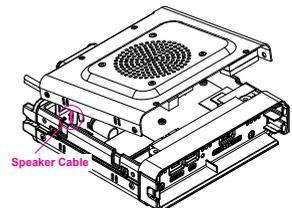
6. Unplug the speaker cables extending from the top cover from the socket on the board inside the main body before removing the cover.
