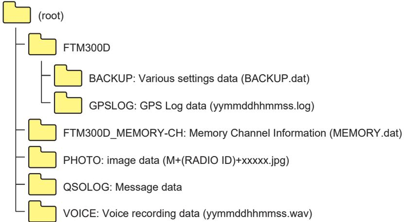
The [yymmddhhmmss] part of the file name consists of year (yy), month (mm), day (dd), hour (hh), minute (mm), and second (ss).
