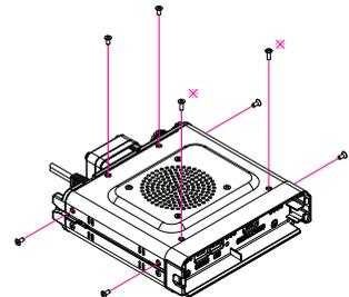
5. Carefully lift the top cover of the main body.
