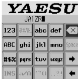
Touch [123] to switch to the numeric input screen. Touch [ABC] in the numeric input screen to return to the alphabet input screen. Press [X] to complete the Call Sign entry.
