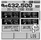
3 Rotate the DIAL, then touch [PICT]. Displays the list of image data saved on the microSD memory card.
