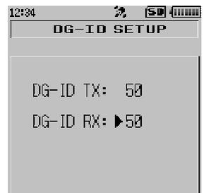
5. Press and hold the **[GM]** key to save the setting and return to normal operation.
