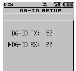
4. Press the **[GM]** key, then rotate the **DIAL** knob to set the receive DG-ID number (DG-ID RX) to “50”.
