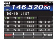
2. Rotate the **MULTI** knob to select the DG-ID "01" memory register to store the TX and RX DG-ID numbers.
