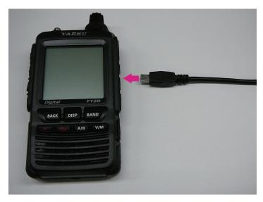
6. While pressing down A/B, connect the AC adaptor connector to the FT2DR/DE EXT DC IN terminal.
