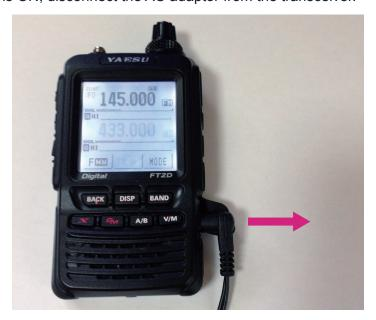
5. Use the supplied cable to connect the FT2DR/DE DATA terminal to the computer.
