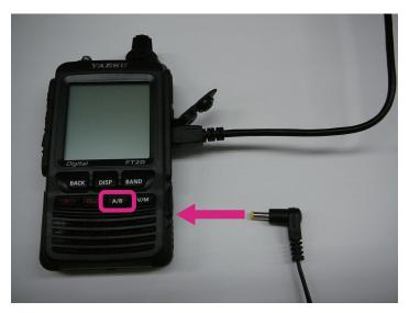
The power turns ON and you will hear a "beep-boop-bop" sound. On the FT2DR/DE display, "---DSP WRITE MODE----" and "Push DISP Key!" will appear.
