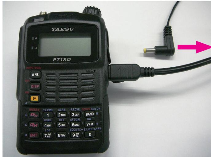
12. Disconnect the cable from the DATA terminal and the computer.
