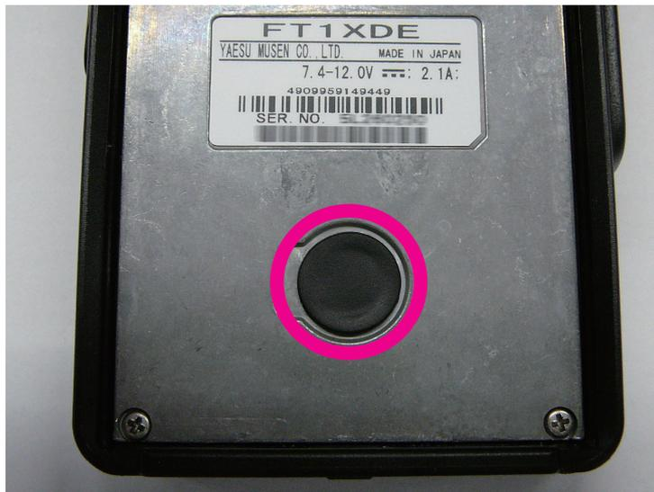
Do not forget to move the program switch at the back of the main body to the normal operating mode position (downward) and then cover up the switch with the rubber cap.
