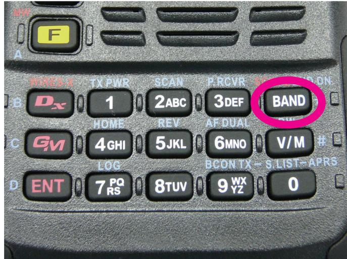
20. When the display lights up fully, press the [BAND] key and check the Version No. displayed.
