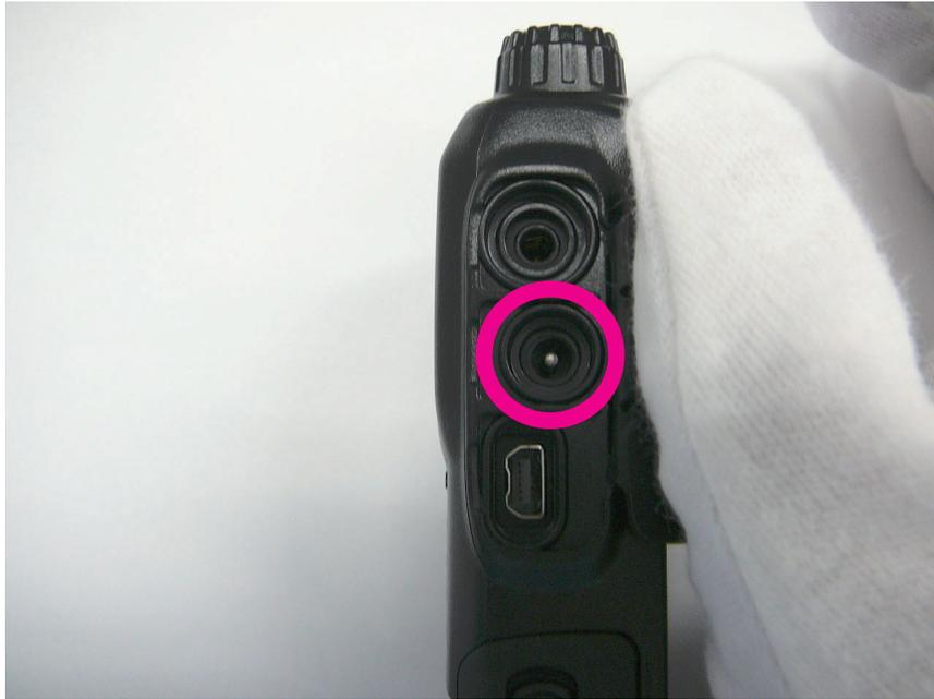
Connect the AC adapter to a wall outlet and then insert the plug to the FT1XDR/DE EXT DC IN terminal.
