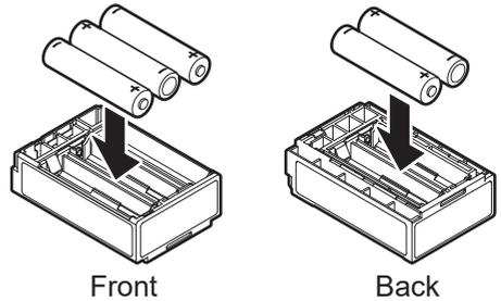
4. Install the **SBT-13** into the battery compartment and align it to the battery contacts until it clicks.
