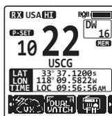
The radio will monitor the priority channel and the watch channel that was selected in step 2.
