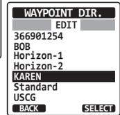
3. Select “NAME” or “POSITION” with the [CH▼]/[CH▲] key, then press the [SELECT] soft key.
