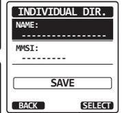
5. Repeat steps 3 and 4 until the name is complete. The name can consist of up to eleven characters, and if you do not use all eleven characters, select "→" to move to the next space. This method can also be used to enter a blank space in the name.
