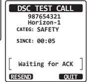
*DSC Test Call by Manually Entering an MMSI*
