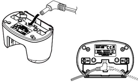
2. Plug the **SAD-25** into the AC line outlet.
