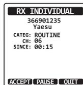
**ACCEPT:** Press this key to accept the DSC individual call and automatically switch to the requested channel.
