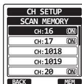
To check channels to be scanned, press the [CH▼]/[CH▲] key repeatedly. The “**MEM**” icon will appear when the memory channel is displayed.
