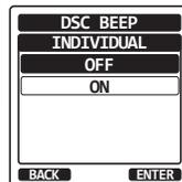
To re-enable the ringer tone, repeat the above procedure, pressing the [CH▼]/[CH▲] key to select “ON” in step 2 above.
