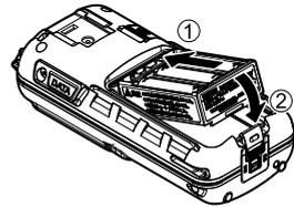
To remove the battery case, turn the transceiver **OFF**, open the battery cover, then push and lift up the bottom end of the battery case.
