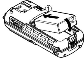
To remove the battery pack, turn the transceiver off, open the battery cover, then push and lift up the bottom end of the battery pack.
