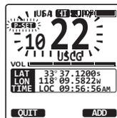
4. Repeat steps 1 through 3 to program all the desired channels into the preset memories. Up to 10 channels can be registered. If you attempt to register the 11th channel, the error beep will sound.
