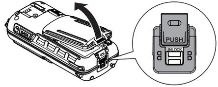
3. Install the **SBR-13LI** battery pack into the battery rest aligning it to the battery contacts until it clicks.
