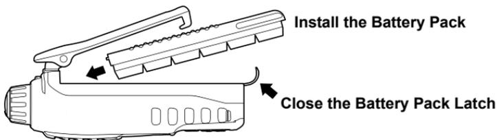
3. To remove, open the Battery Pack Latch on the bottom of the transceiver, then slide the battery downward and out from the transceiver.
