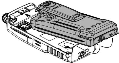
To remove the battery, turn the radio off. Slide the Battery Pack Latch on the bottom of the radio, then lift up on the bottom of the battery and remove it from the radio.
