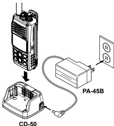
**NOTE:** The green LED indicator may blink after charging is complete, but this is not a malfunction.
