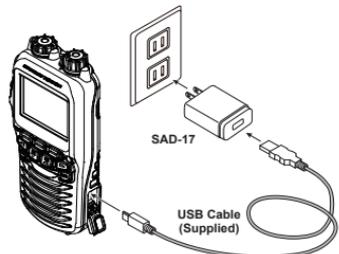
4. If the connection is correct, the **RAM4W**'s LCD display will show the battery-charging icon.
