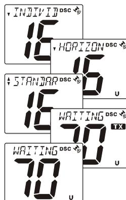
If the reply signal is not received, the transceiver will transmit again.
