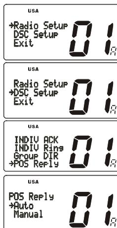
The **GX3500S** has the capability to turn off the Position Request ringer.
