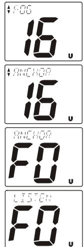
To exit from the FOG HORN mode, press and hold down the [NAV] key again.
