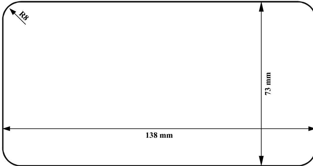
**Use this template to mark the location where the rectangular hole for the flush mount is to be cut.**
