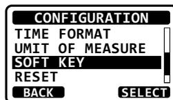
6. Press the **▲ / ▼** keys to select how long the soft key icon will be shown on the display after a soft key is pressed, then press the **ENTER** soft key.
