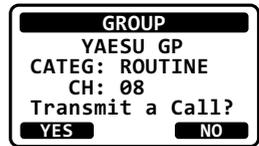
8. After the group call is transmitted, the transceiver will switch to the channel selected in step 6 above, without changing the display. To change the display, press the **QUIT** soft key.
