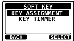
7. Press the **▲ / ▼** keys to select the desired key function, then press the **ENTER** soft key. Refer to the next page for available functions.
