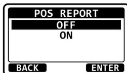
To enable the position report ringer, repeat the above procedure, pressing the **▲ / ▼** keys to select “ON” in step 7 above.
