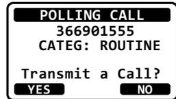
10. After the polling call is transmitted, the **GX1300** waits for a reply from the radio which was called, and the display will show “WAITING FOR ACK”.
