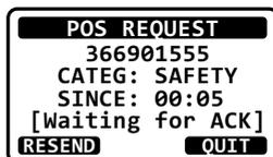
11. When the **GX1300** receives the position from the polled vessel, the **GX1300** will produce a ringing alarm sound and the position from the polled vessel is sent to a GPS chart plotter via NMEA 0183. (DSC BEEP needs to be enabled to hear alarm.)
