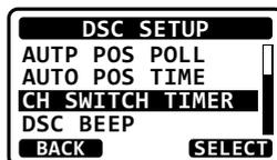
5. Press the **▲ / ▼** keys to select the desired time, then press the **ENTER** soft key. The switching time can be set to “OFF”, “10 sec”, “30 sec”, “1 min”, or “2 min”.
