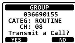
11. After the group call is transmitted, the transceiver will switch to the channel selected in step 9, without changing the display. To change the display, press the **QUIT** soft key.
