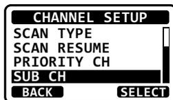
7. Press the **BACK** soft key to exit the menu and return to radio operation.
