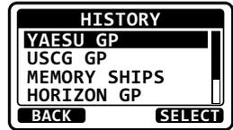
6. Press the ▲ / ▼ keys to select the operating channel you want to communicate on and press the **SELECT** soft key.
