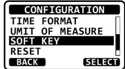
6. Press the **▲ / ▼** keys to select the desired soft key number, then press the **SELECT** soft key.
