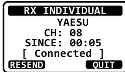
8. Monitor the channel to make sure it is clear, then press the **PTT** switch on the microphone and talk to the calling vessel.
