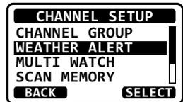
7. Press the **BACK** soft key to exit the menu and return to radio operation.
