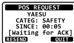
8. When the **GX1300** receives the position from the polled vessel, the **GX1300** will produce a ringing alarm sound and the position from the polled vessel is sent to a GPS chart plotter via NMEA 0183. (DSC BEEP needs to be enabled to hear alarm.)
