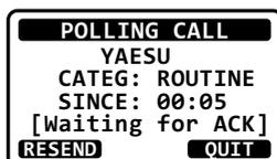
8. When an acknowledgement signal is received, the display will show “Received ACK”.
