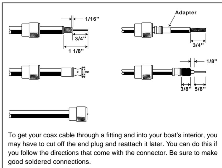
To get your coax cable through a fitting and into your boat's interior, you may have to cut off the end plug and reattach it later. You can do this if you follow the directions that come with the connector. Be sure to make good soldered connections.
