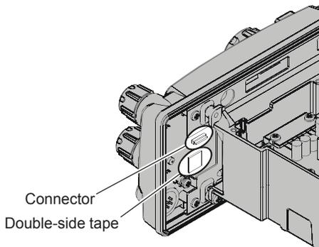
3. Carefully align the connector on the **BU-1** with the connector on the Printed Circuit Board, and gently press the **BU-1** into place.
