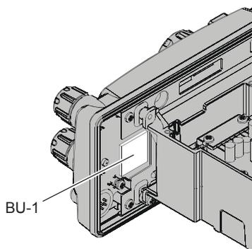
4. Replace the Rear Case, using the screws and washer removed in the first step.
