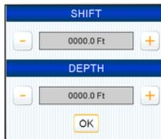
The range window allows to adjust the Shift and Depth value. Tap on the relative **+** or **-** to reach the desired value, than tap on **OK** (the Range window disappears).
