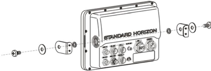
5. Slide the CPN Series Chart Plotter into the dash of mounting hole.
