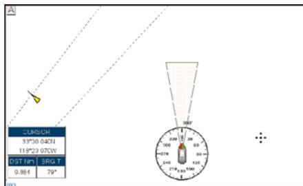
Figure 13.3 - Grounding Alarm on CPF300i
