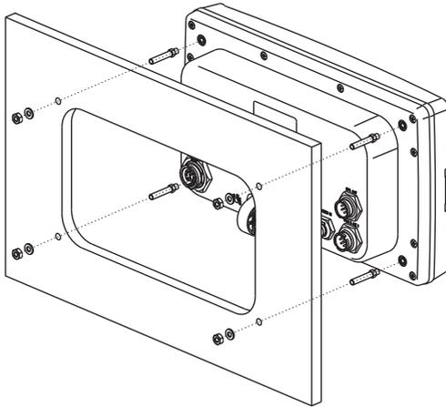
Figure 2.2a - Example of Flush installation on CPF300i
