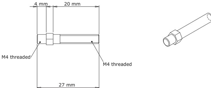
Figure 2.2.0 - Mounting Screws
