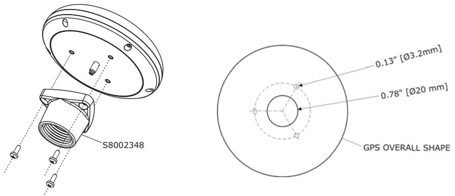
Figure 2.3.0 - Installing the External GPS antenna (I)
