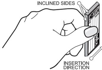
Figure 5.0 - Inserting C-CARD
