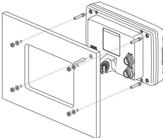
Figure 2.2 - Example of Flush installation on CPF180i
