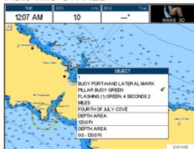
**CURSOR WINDOW** By default when the cursor is moved on the chart a window is shown with the Lat/Lon Distance and Bearing from the vessels location to the cursor. This selection allows the window to be turned On (default) or Off. The Cursor Window is automatically disabled when General is set in Windows Setup option.
