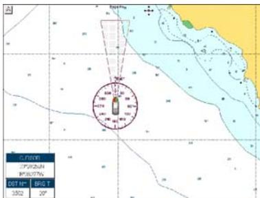
Figure 13.3 - Grounding Alarm
