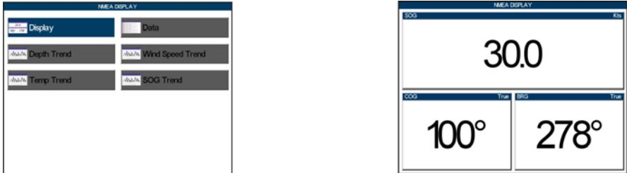
Figure 12.6 - NMEA Display menu (on the left) and default NMEA Display page (on the right)
