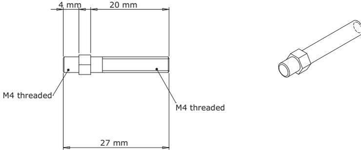
Figure 2.2.0 - Mounting Screws
