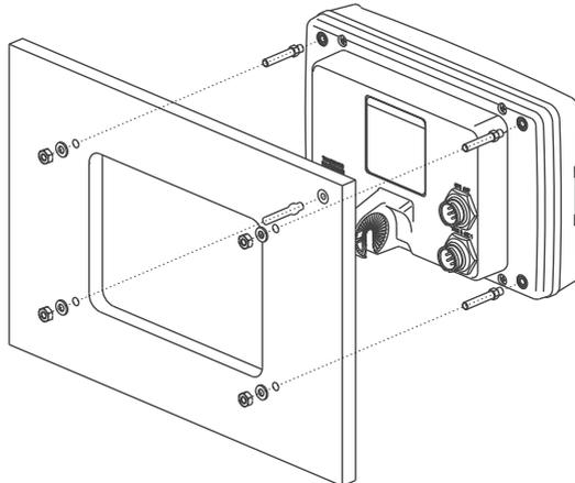
Figure 2.2 - Example of Flush installation on CPF190i
