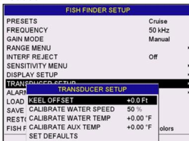
Figure 17.12 - Transducer Setup menu
