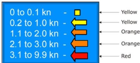
When the GPS Chart Plotter receives a valid position fix, the Tide icons are shown on the charts on the basis of the current date and time: the screen displays and changes arrows as date/time changes.
