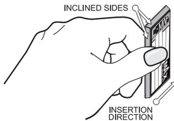
Figure 5.1 - Inserting C-CARD
