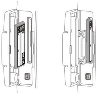
Figure 5.1a - Inserting C-CARD (details)
