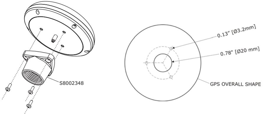
Figure 2.3.0 - Installing the External GPS antenna
