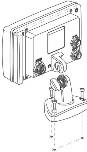
Figure 2.1 - Example of Bracket installation on CPF190i
