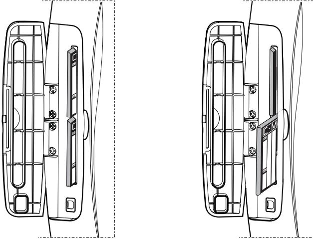
Figure 2.7a - Inserting C-CARD (II)
