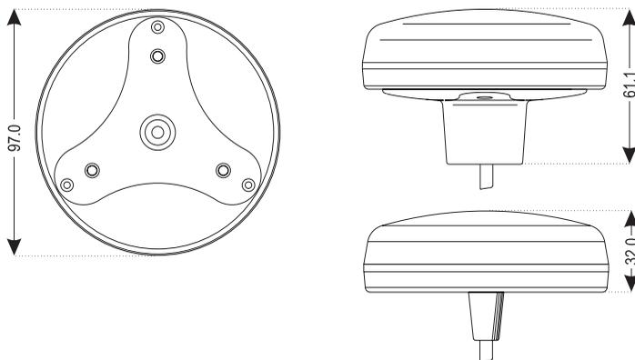
Figure 2.1.1 - Smart DGPS WAAS antenna Dimensions
