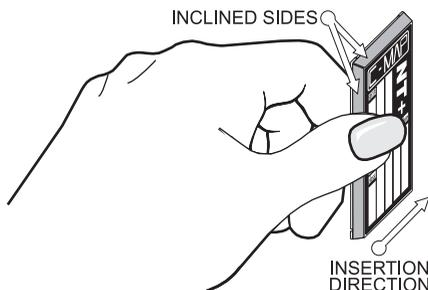
Figure 2.7 - Inserting C-CARD (I)
