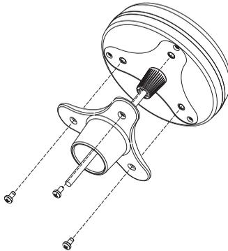
**Figure 2.1 - Installing the Smart DGPS WAAS antenna (I)**
