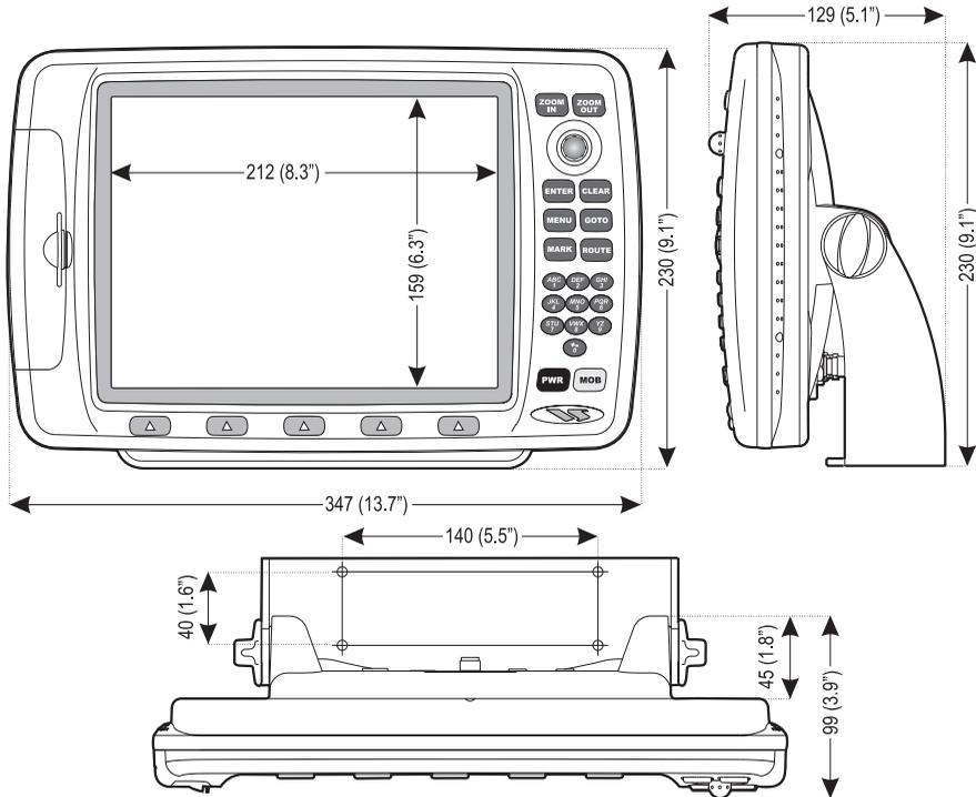
Figure2.0.0 - Chart plotter Dimensions [mm/inch]
