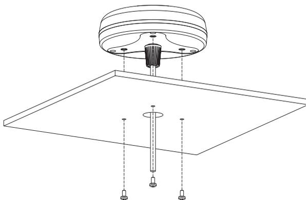
Figure 2.1b - Installing the Smart DGPS WAAS antenna (III)
