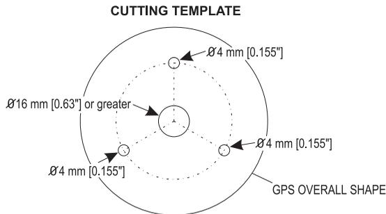
**Figure 2.1a - Installing the Smart DGPS WAAS antenna (II)**
