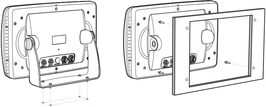
Figure 2.0 - Installing/removing chart plotter
