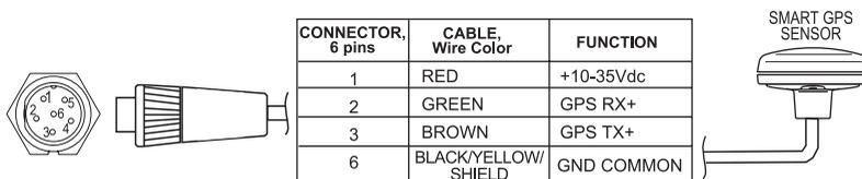
Figure 2.1.0 - GPS Cable wires description
