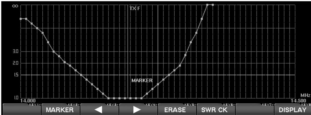
1. Press the [F2](**MARKER**) key to turn the marker function on; the marker cursor will be displayed.
