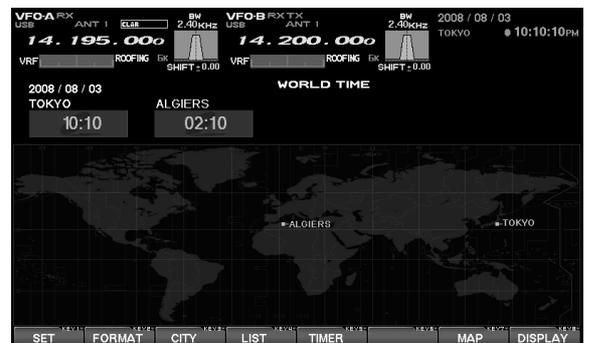
**Note:** The [F1](SET) key is only used when setting the city name and local time. If you make a mistake, press the [F7](SELECT) key momentarily. Pressing the [F7](SELECT) key for two seconds will return you to the World Map screen.
