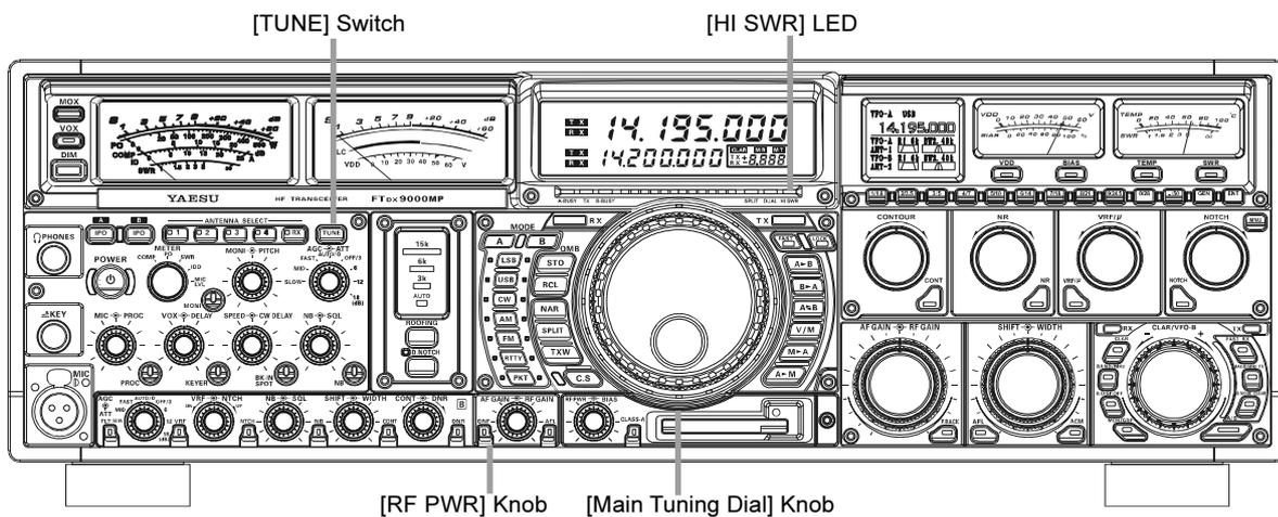
1. Rotate the **[RF PWR]** control (fully clockwise (to the right)).
