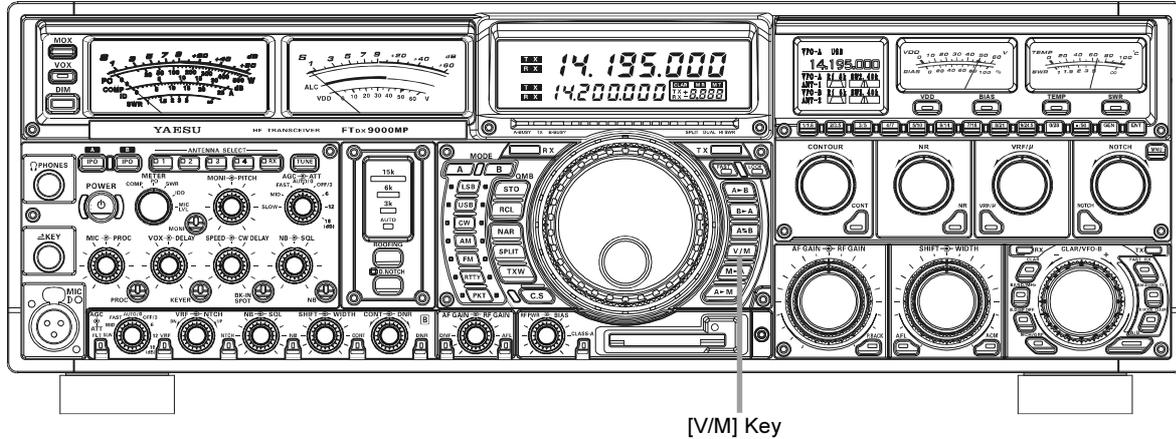
1. Press the **[V/M]** key once to enter the “Memory” mode (a memory channel number “USX” will appear on the display in the Multi-Panel in the Frequency display).
