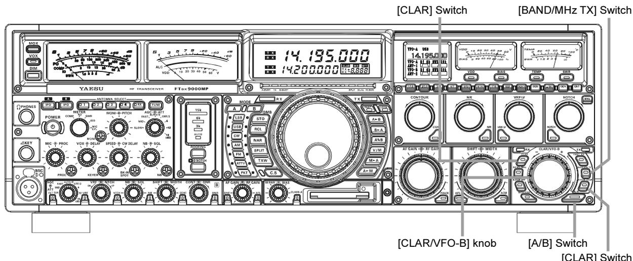
1. Press the **[CLAR]** switch. The Red LED imbedded in the switch will light up, and “**CLAR**” will appear in the Multi Panel Window on the Frequency Display. The **[CLAR/VFO-B]** knob will now be enabled for offset tuning of the transmitter.
