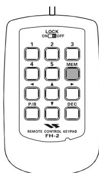
4. Press the FH-2's [1] ~ [5] key to select the desired Message Memory Register into which you wish to program the text.
