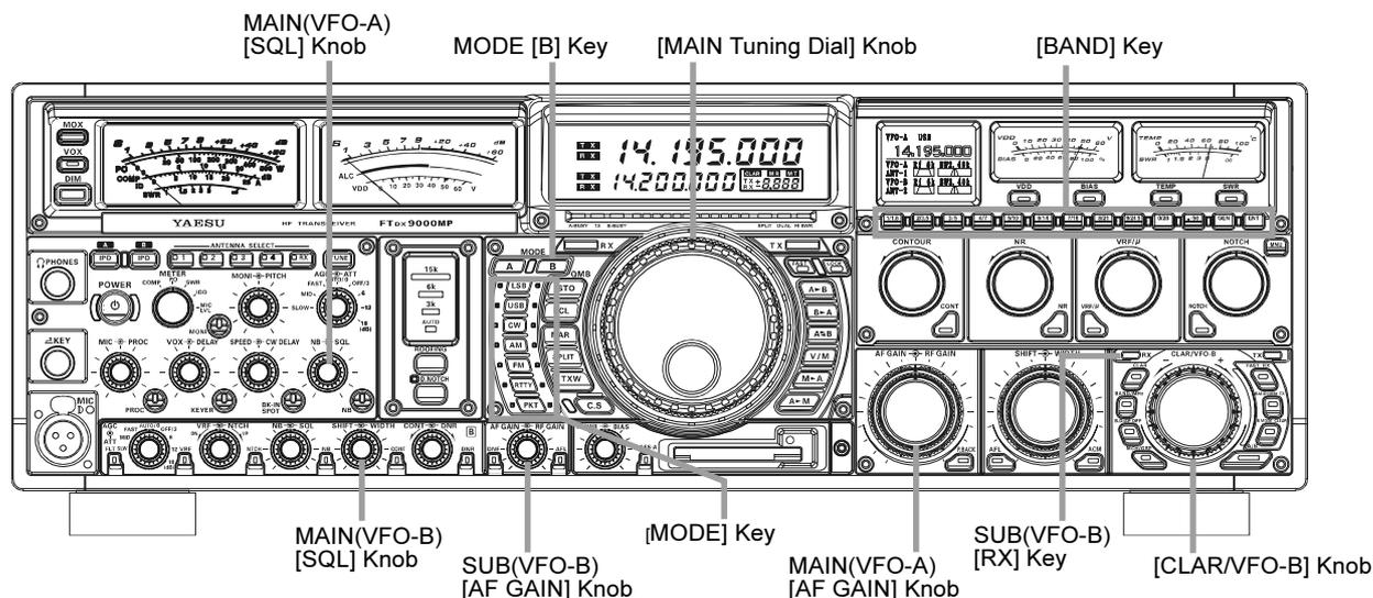
1. While receiving on the Main band (VFO-A), engage the Sub (VFO-B) receiver by pressing the Sub **[RX]** key. You will now be receiving on the two frequencies shown on the main frequency display.
