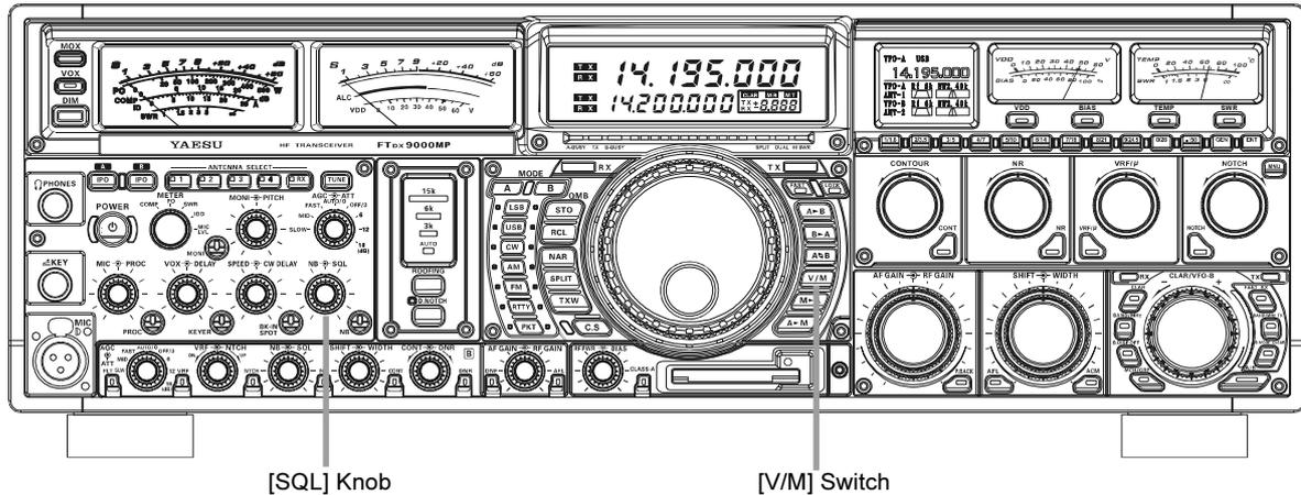
1. Set the transceiver up in the memory mode by pressing the **[V/M]** key, if necessary.
