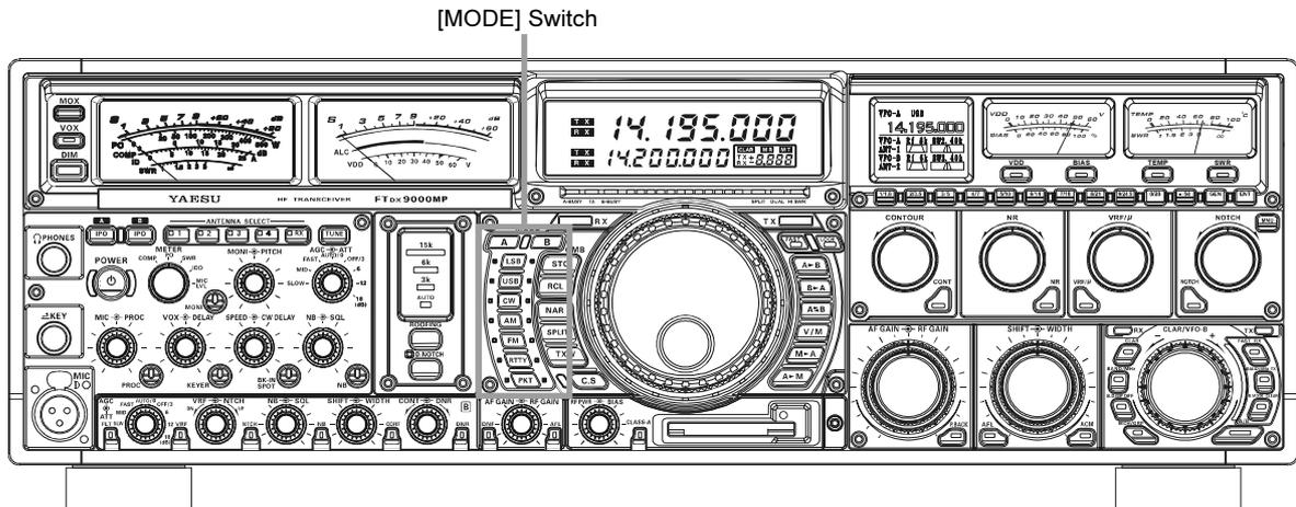
1. To start, let's use a typical example where you have set the CW mode (using the default "USB" injection) onto the Main (VFO-A) receiver.
