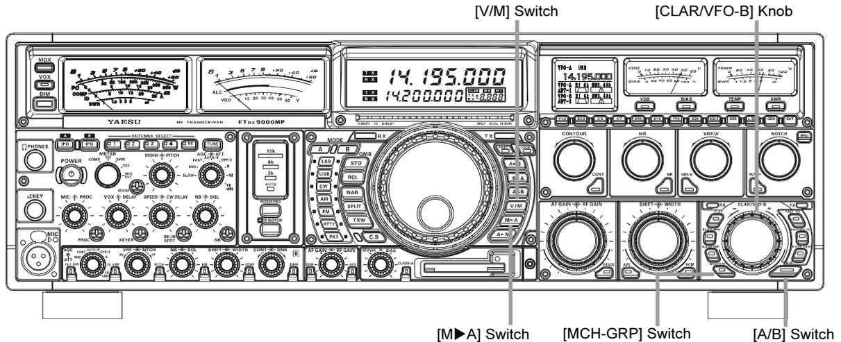
1. Press the **[V/M]** switch, as necessary, to go to the Memory mode. The memory channel number will appear in the multi-panel window.
