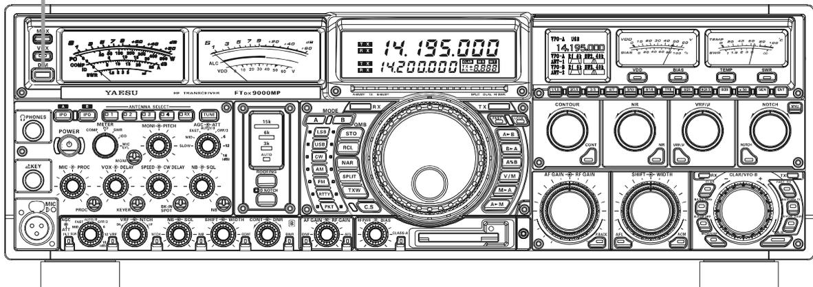
To reduce the illumination level, press the **[DIM]** switch, located to the left of the leftmost analog meter. To restore full brightness, press the **[DIM]** switch once more.
