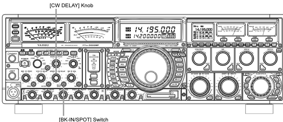
1. Press the [**BK-IN/SPOT**] key momentarily to enable CW transmission (Menu item “**MODE-CW 052 CW BK-IN**” must be set to “SEMI”).
