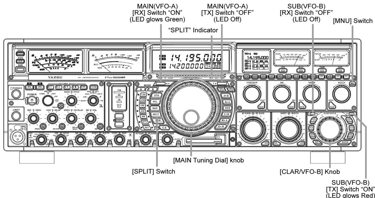
1. Start with regular transceiver operation on the Main (VFO-A) band.
