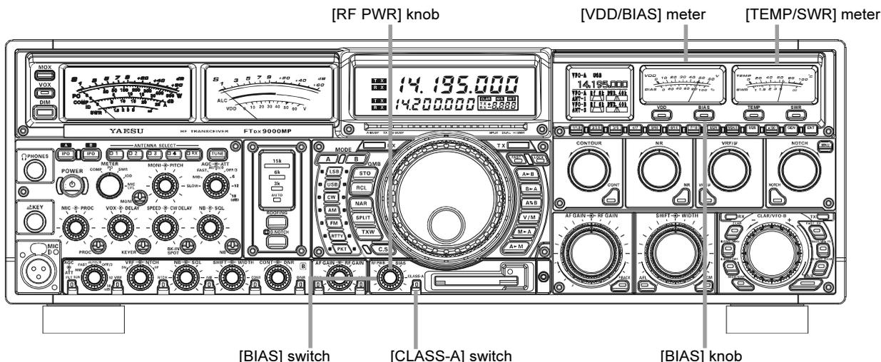
1. To engage Class-A operation, press the **[CLASS-A]** switch. The imbedded Red LED will light up, confirming that Class-A operation has been selected.
