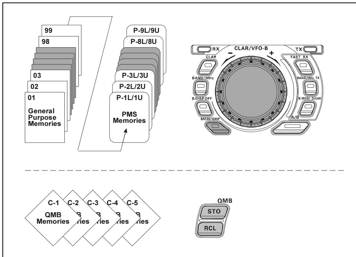
The Quick Memory Bank is comprised of five memories (labeled “C1” ~ “C5”) independent from the regular and PMS memories. These can quickly store operating parameters for later recall.
