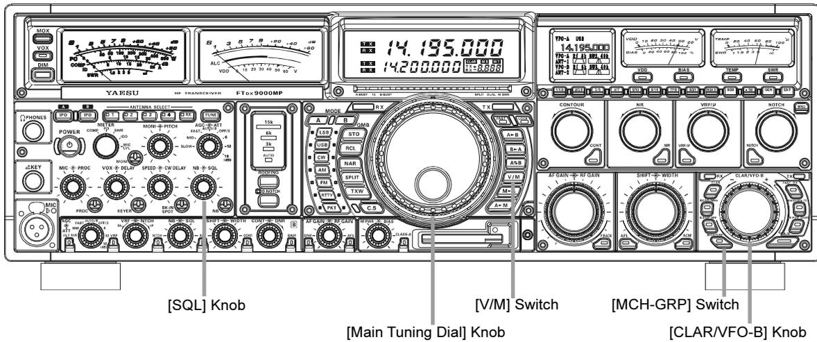
1. Store the Lower and Upper tuning/scanning limit frequencies into the memory pair “P1L” and “P1U,” respectively, or any other “L/U” pair of memories in the special PMS memory area. See page 127 for details regarding memory storage.
