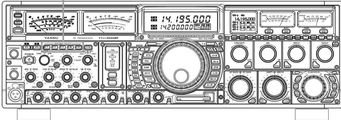
Selection of the desired TX/RX antenna is accomplished by pressing the appropriate [1] ~ [4] Antenna Selection switch on the front panel.
