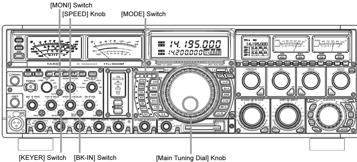
1. Press the **[CW]** mode switch to engage CW operation. If you press the **[CW]** key once more, after initially selecting CW, you will engage the “CW Reverse” mode (see page 113), whereby the “opposite” sideband injection is used, compared to the “normal” sideband. The CW LED will blink for three seconds if you select CW Reverse.
