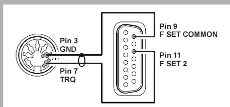
Please cut off the RCA connector on one end of the **CONTROL** Cable supplied with the **VL-1000**, and install a 7-pin DIN connector in its place, according to the illustration.
