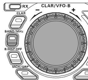
When tuning in 1 MHz steps, clockwise rotation of the [CLAR/VFO-B] knob will increase the frequency, while counter-clockwise rotation will decrease the frequency.
