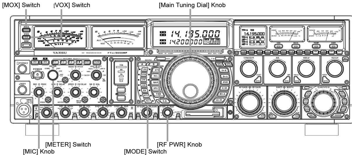
1. The operating mode is selected using the **[MODE]** switches to the left of the **[MAIN Tuning Dial]** knob, and the VFO (A or B) to which the selection is applied is selected by pressing the **[A]** or **[B]** switch above the Mode keys. Press the **[A]** or **[B]** key to select the desired VFO, then press the **[LSB]** or **[USB]** key to select one of the SSB modes. For AM operation, press the **[AM]** key.
