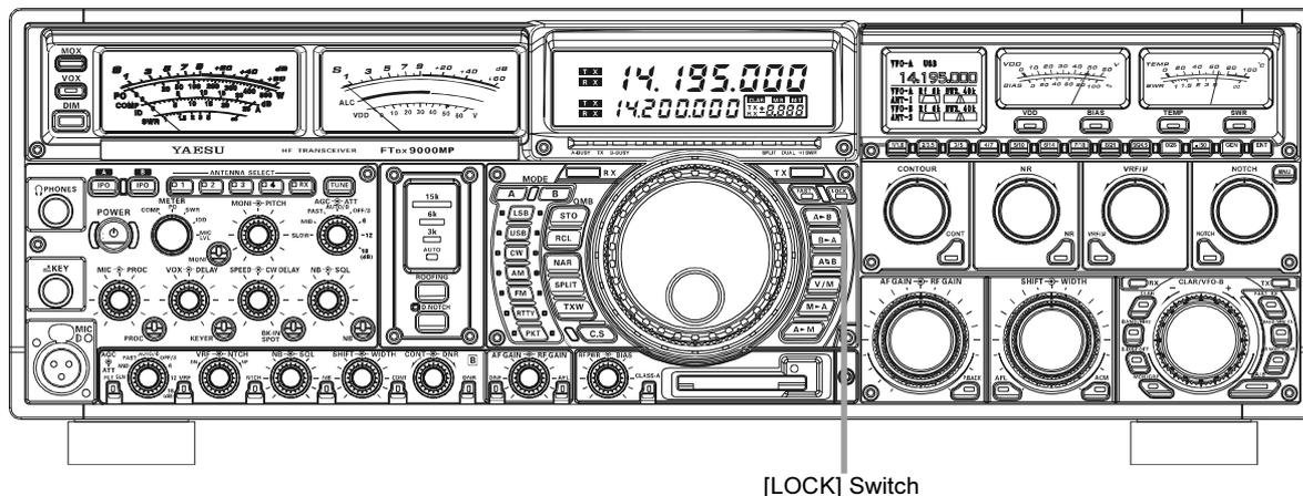
To lock out the [MAIN Tuning Dial] knob, just press the [LOCK] switch that is located to the right of the Dial. To unlock the Dial setting, and restore normal tuning, just press the [LOCK] switch once more.
