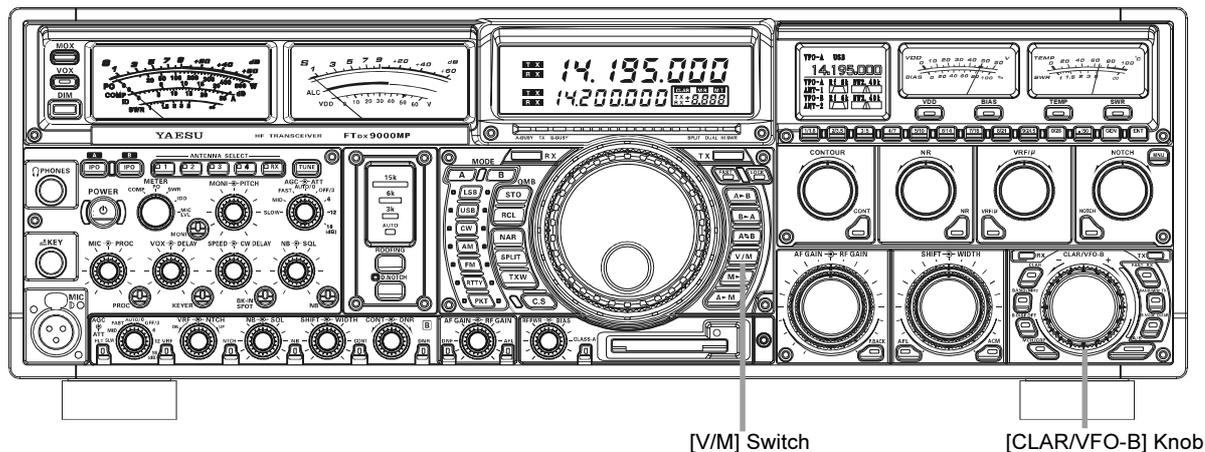
To operate on the 60-meter band channels, press the **[V/M]** key, if necessary, to enter the Memory mode, then rotate **[CLAR/VFO-B]** knob to select the desired channel from the above selections.
