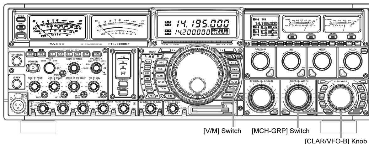
1. Press the **[V/M]** key, if necessary, to enter the Memory mode.
