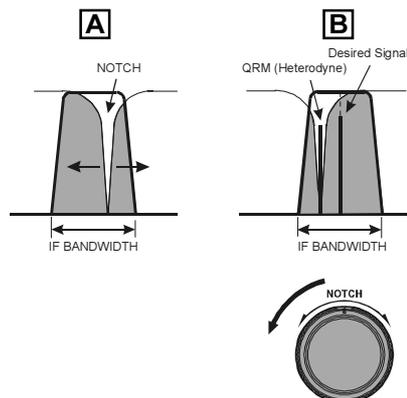
To switch the IF Notch filter off, press the Sub (VFO-B) band's **[NTCH]** switch once more. The LED imbedded in the switch will turn off, confirming that the IF Notch filter is no longer operating.
