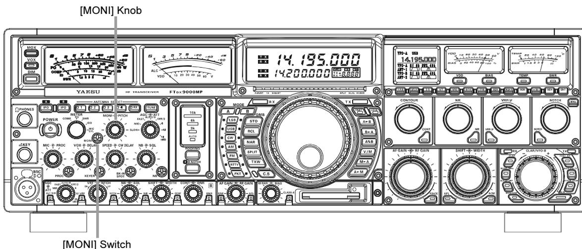
1. Press the **[MONI]** switch. The imbedded Red LED will light up, indicating that the Monitor is turned on.
