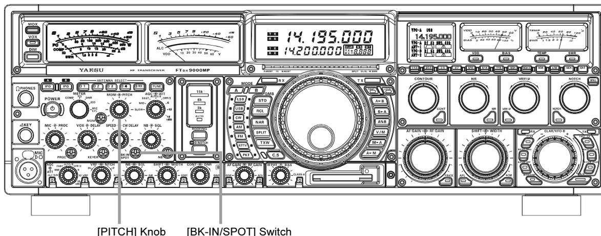
For everyday operation, the (CW) [PITCH] control allows you to set the center of the receiver passband, as well as the offset pitch of your CW carrier signal, to the tone pitch you prefer to listen to.
