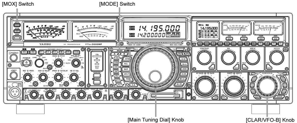
1. Rotate the **[MAIN Tuning Dial]** knob to the output frequency (downlink) from the repeater.
