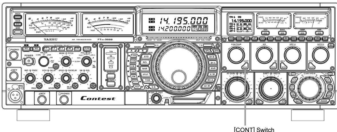
Press and hold the **[CONT]** switch for 2 seconds to activate the Audio Peak Filter (APF) circuit. The LED inside the **[CONT]** switch will blink amber for 3 seconds, then replaces to continuous glow. The APF is an automatic circuit, and there is no adjustment knob for the APF.
