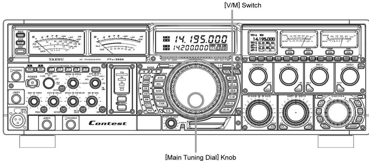
1. Press the **[V/M]** switch to recall any memory channel.
