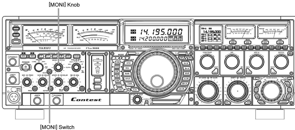
1. Press the **[MONI]** switch. The imbedded Red LED will light up, indicating that the Monitor is turned on.
