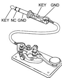
3. Press the **[BK-IN/SPOT]** key momentarily to engage automatic activation of the transmitter when you close the CW key. The LED imbedded in the **[BK-IN/SPOT]** switch will light up.
