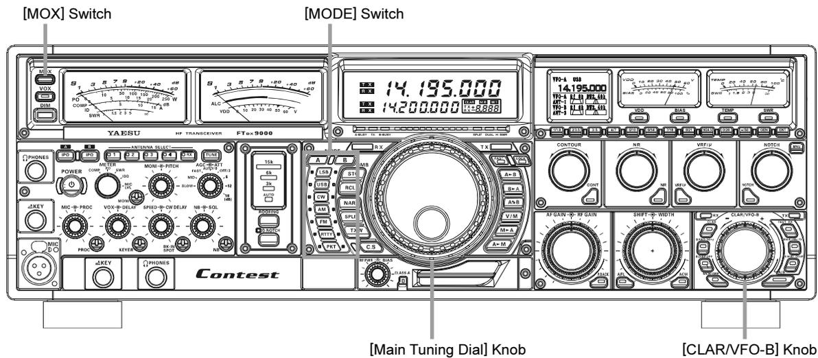
1. Rotate the **[Main Tuning Dial]** knob to the output frequency (downlink) from the repeater.
