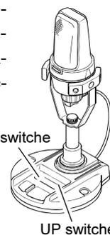
The microphone’s **[UP]/[DOWN]** switches utilize the tuning steps of the **[Main Tuning Dial]** knob; moreover, when the microphone’s **[FAST]** key is pressed, the tuning rate increases by a factor of ten, in a manner similar to the effect of the transceiver’s front-panel **[FAST]** key.
