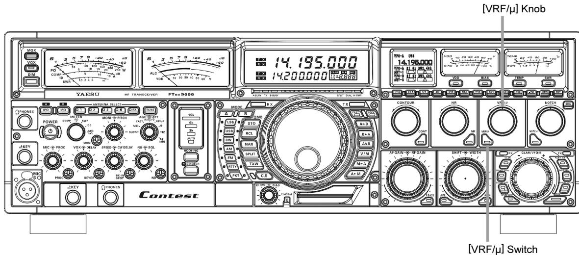
1. Press the **[VRF/μ]** switch momentarily. The LED inside the switch will become illuminated, and the VRF system will be engaged, centered on your current Amateur band.
