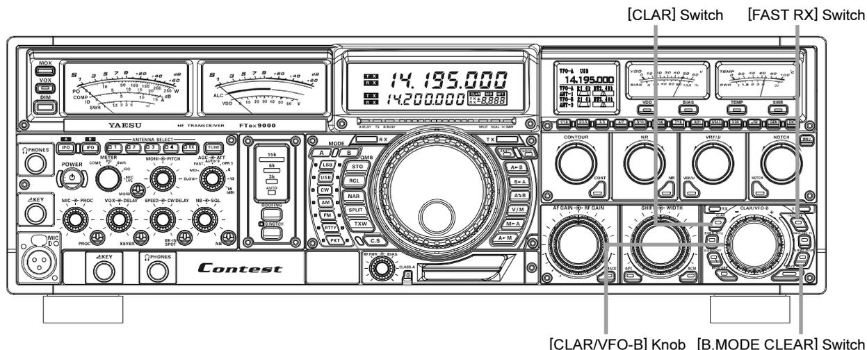
1. Press the [CLAR] switch. The LED imbedded in the switch will glow Red to signify that rotation of the [CLAR/VFO-B] knob will allow setting of a frequency offset.
