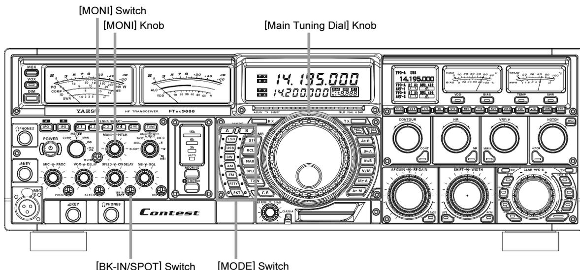
1. Press the **[CW]** mode switch to engage CW operation.
