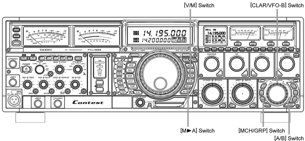
1. Press the **[V/M]** switch, as necessary, to go to the Memory mode. The memory channel number will appear in the multi-panel window.
