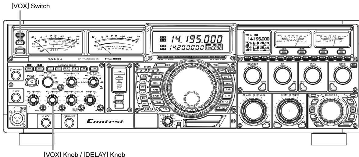
1. To start, set the **[DELAY]** and **[VOX]** controls fully counter-clockwise (to the left).
