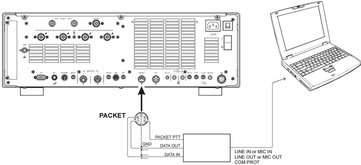
Use the “Packet” mode for AFSK-based Baudot and other data modes.
