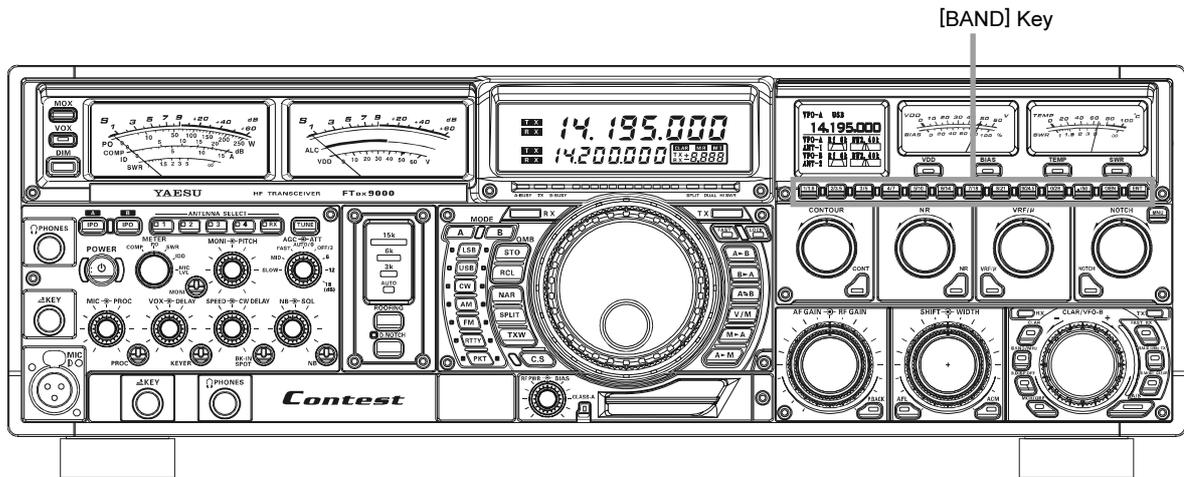
1. Press and hold in the **[ENT]** key (one of the **[BAND]** keys) for two seconds. The frequency display area will change over to the “Rotator Control” configuration.
