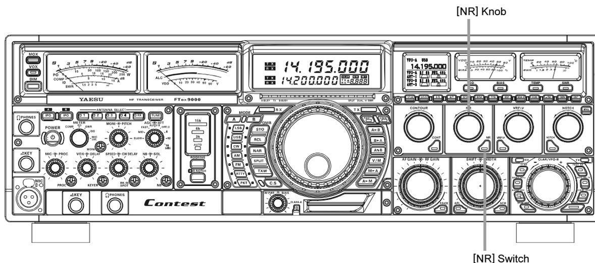
1. Press the [NR] switch. The LED imbedded in the switch will glow Red, confirming that the DNR system is engaged.
