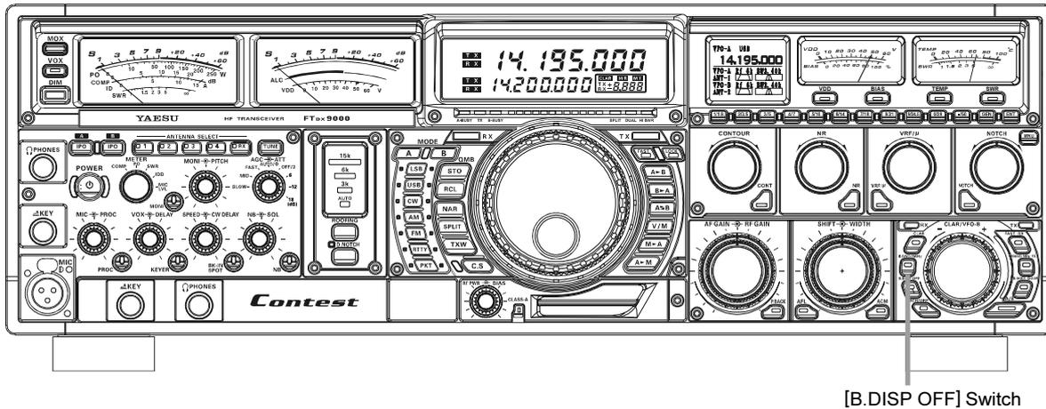
To do this, press the **[B.DISP OFF]** switch, found at the lower left side of the **[CLAR/VFO-B]** knob.
