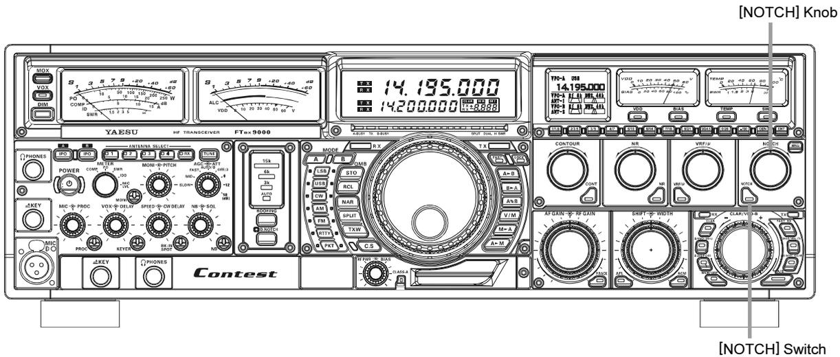
1. Press the **[NOTCH]** switch. The LED imbedded in the switch will glow Red to confirm that the IF Notch filter has been engaged.
