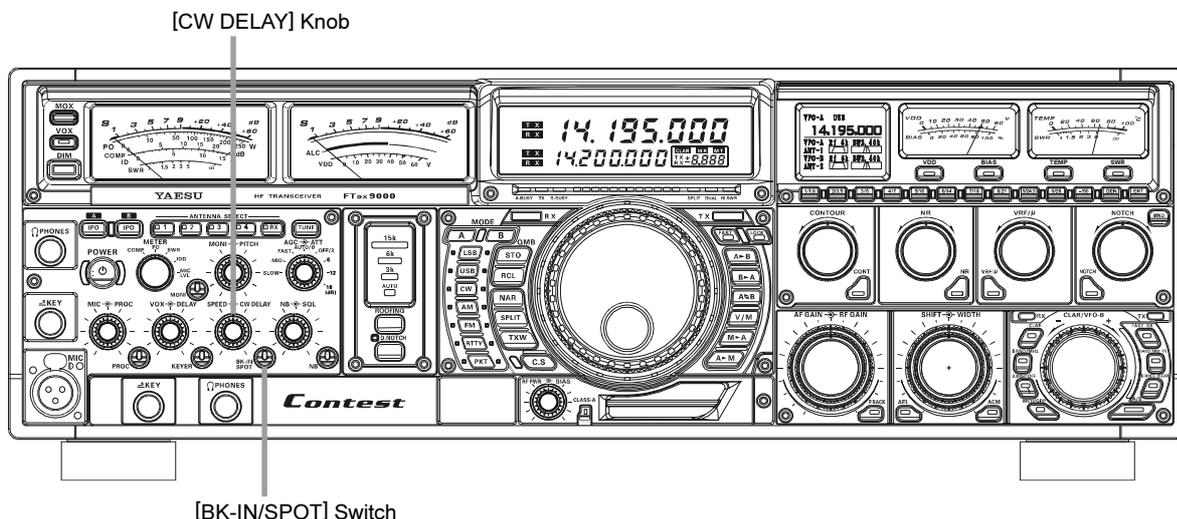
1. Press the [**BK-IN/SPOT**] key momentarily to enable CW transmission (Menu item “**MODE-CW 055 CW BK-IN**” must be set to “**SEMI**”).
