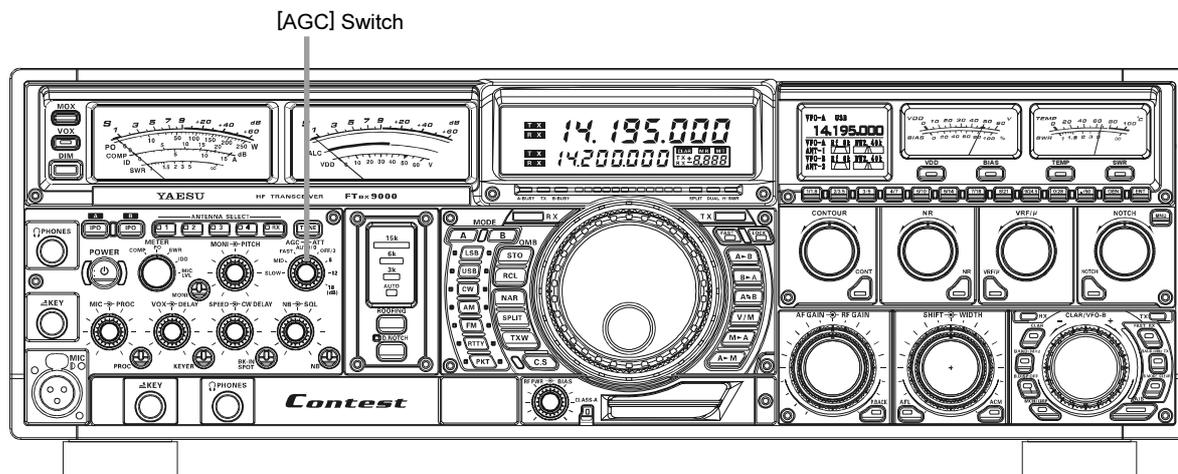
Rotate the **[AGC]** switch to select the desired receiver-recovery time constant. For most operation, we recommend the “AUTO” mode.
