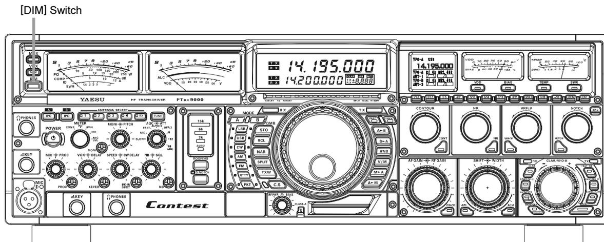
To reduce the illumination level, press the **[DIM]** switch, located to the left of the leftmost analog meter. To restore full brightness, press the **[DIM]** switch once more.
