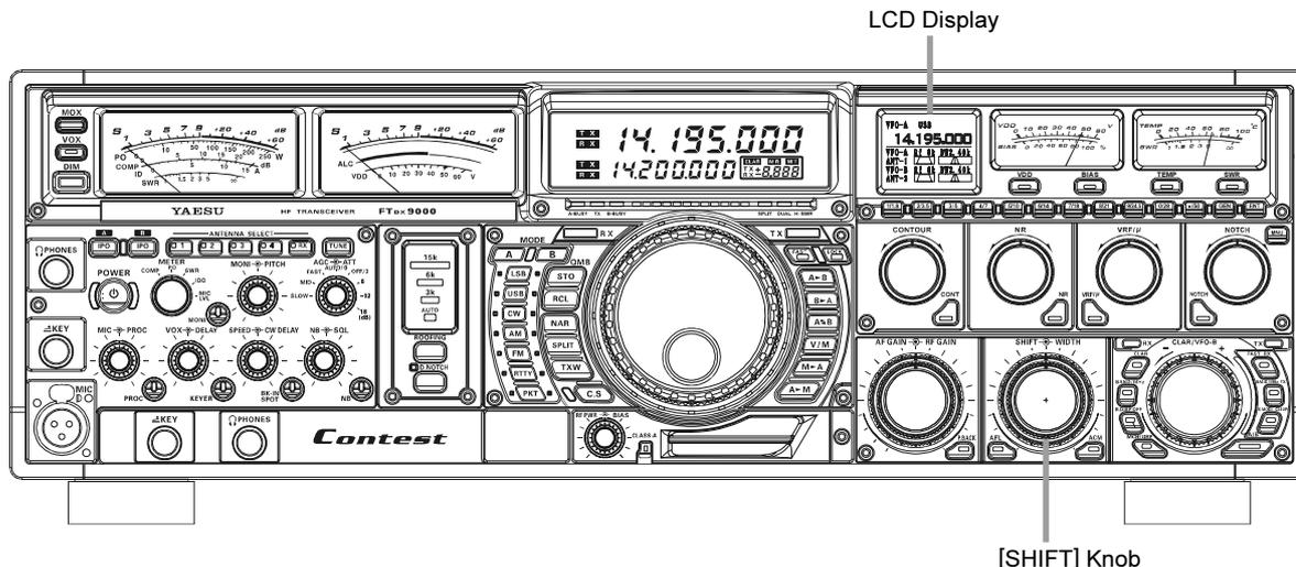
Rotate the **[SHIFT]** control to the left or right to reduce the interference.
