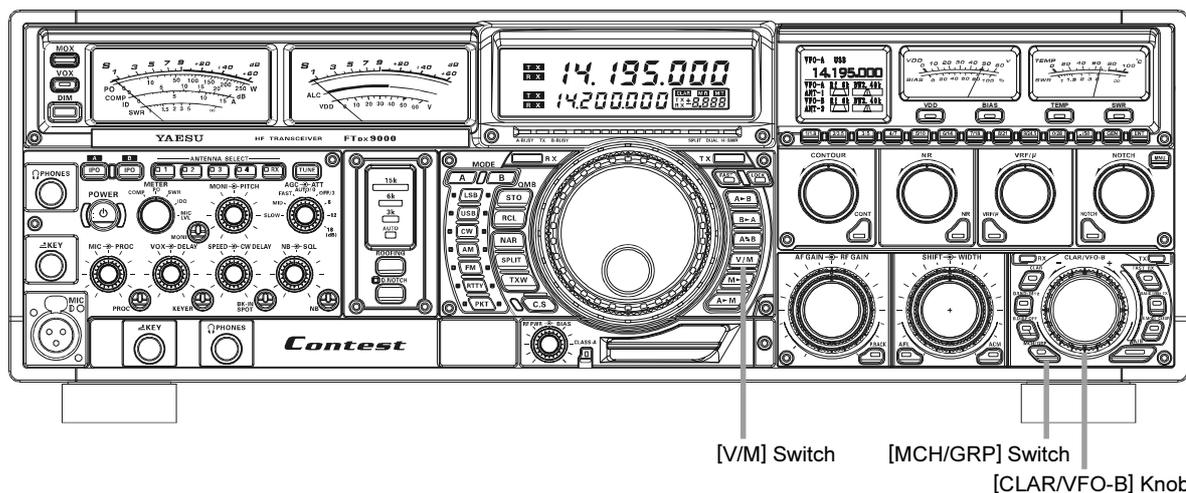
1. Press the **[V/M]** key, if necessary, to enter the Memory mode.
