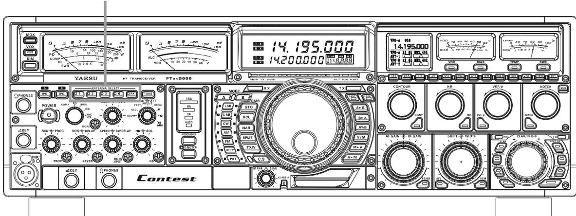
Selection of the desired TX/RX antenna is accomplished by pressing the appropriate [1] ~ [4] Antenna Selection switch on the front panel.
