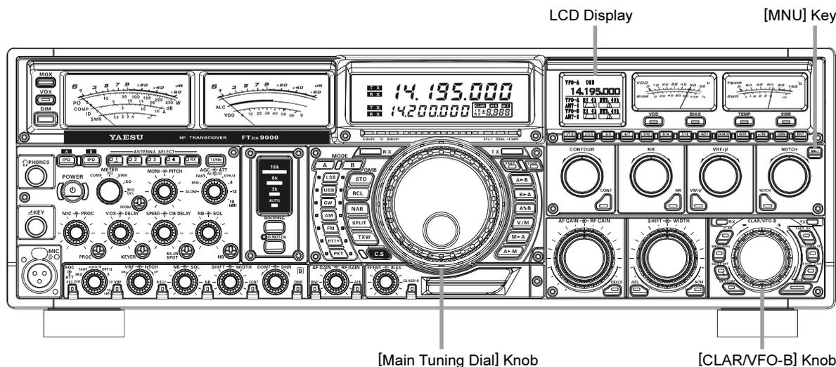
1. Press the [MNU] key to engage the Menu mode; the Menu list will appear on the LCD Display.
