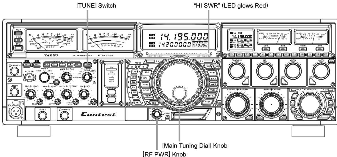
1. Rotate the **[RF PWR]** control fully clockwise (to the right).
