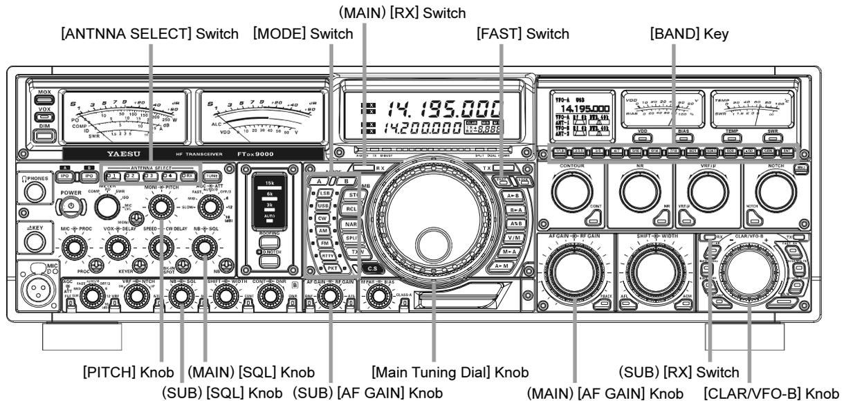
1. While receiving on the VFO-A, engage the VFO-B by pressing the **[SUB RX]** key. You will now be receiving on the two frequencies shown on the main frequency display.
