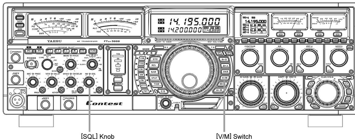
1. Set the transceiver up in the memory mode by pressing the [V/M] switch, if necessary.
