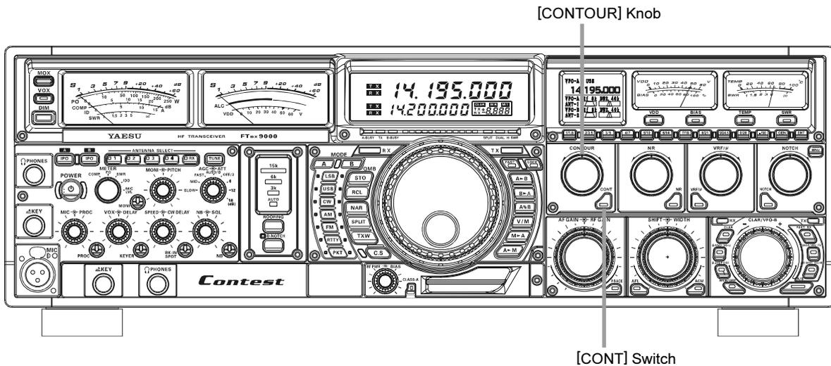
1. Press the **[CONT]** switch. The LED imbedded in the switch will glow Red to confirm that the Contour filter is engaged.
