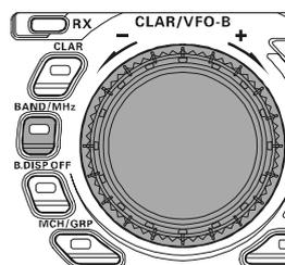
When tuning in 1 MHz steps, clockwise rotation of the **[CLAR/VFO-B]** knob will increase the frequency, while counter-clockwise rotation will decrease the frequency.
