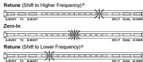
※: When the CW reverse feature is activated, the indication of the Tuning Offset Indicator is oppositely
