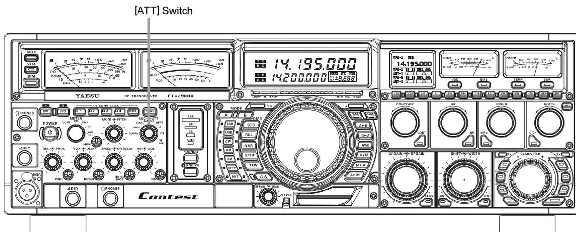
Rotate the **[ATT]** switch to set the desired attenuation level, per the chart below.
