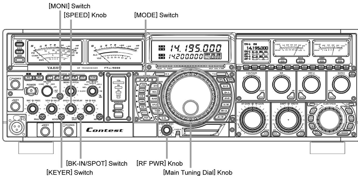
1. Press the **[CW]** mode switch to engage CW operation.
