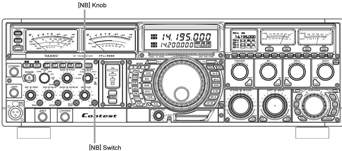
1. Press the **[NB]** switch momentarily to reduce a short pulse noise such as from switching transients, automobile ignitions and power lines. The LED imbedded in the switch will glow Red to confirm that the Narrow-NB is operating. Press and hold the **[NB]** switch for 2 seconds to reduce a longer duration man-made pulse noise. The LED imbedded in the switch will glow Yellow to confirm that the Wide-NB is operating.
