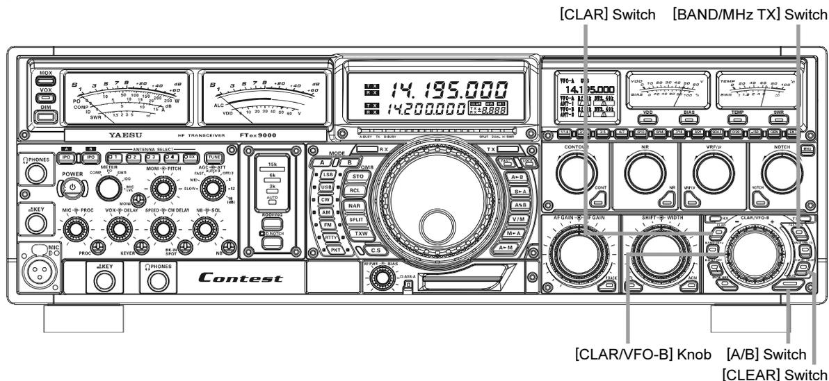
1. Press the **[CLAR]** switch. The Red LED imbedded in the switch will light up, and “CLAR” will appear in the display. The **[CLAR/VFO-B]** knob will now be enabled for offset tuning of the transmitter.
