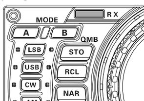
5. Press the [A] switch to enable the capability to change the operation for the VFO-A the imbedded LED will glow Red.
