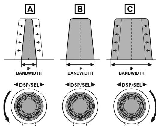
**Mode SSB:** 1.8 kHz / 2.4 kHz / 3.0 kHz
