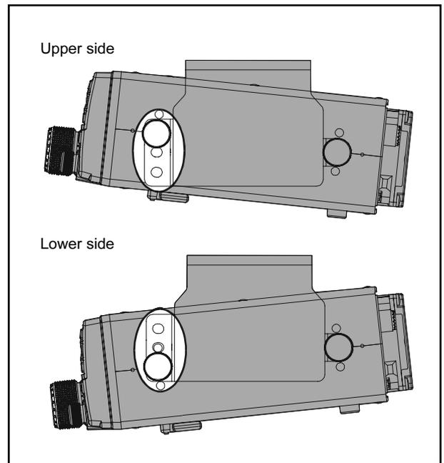
2. Position the transceiver in the bracket so the holes in the side are aligned with those in the bracket. Fasten the transceiver into place using the supplied Knob-screws (M4).
