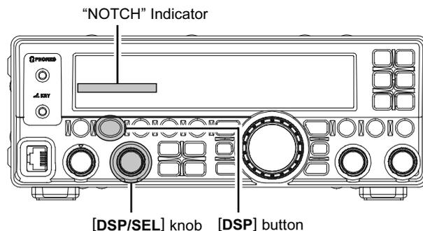
The performance of the IF Notch filter is shown in Figure “A”, where the effect of rotation of the **[DSP/SEL]** knob is depicted. In Figure “B”, you can see the notching effect of the IF Notch filter as you rotate the **[DSP/SEL]** knob to eliminate the incoming interference.
