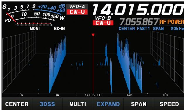
**Figure 4** — The **3DSS** setting changes the spectrum scope to a three-dimensional view with signals marching off the back of the screen over time. A standard waterfall display is available when the 3D view is deactivated.
