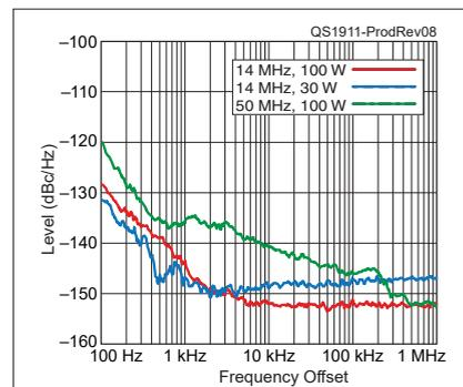
**Figure 8** — Spectral display of the Yaesu FTdx101D transmitter output during phase-noise testing. Power output is 100 W on the 14 MHz band (red trace), 30 W on the 14 MHz band (blue trace), and 100 W on the 50 MHz band (green trace). The carrier, off the left edge of the plot, is not shown. This plot shows phase noise 100 Hz to 1 MHz from the carrier. The reference level is -100 dBc/Hz, and the vertical scale is 10 dB per division.
