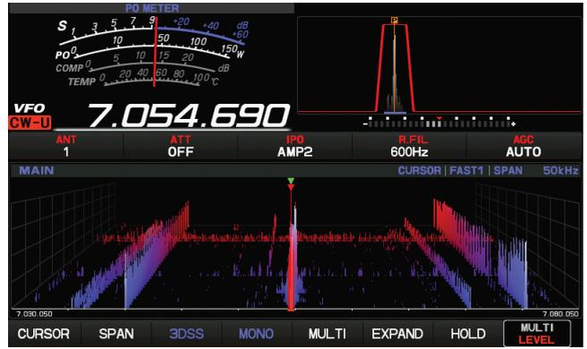
**Figure 2** — Same as Figure 1, except we have tapped the 3DSS on-screen button and now have a three-dimensional view with time marching out the back of the screen, instead of the waterfall. This way, you can see what happened before, as well as what’s happening now.
