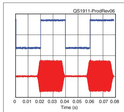
**Figure 6** — CW keying waveform for the Yaesu FTdx101D showing the first two dits in full-break-in (QSK) mode using external keying and the default rise time setting. Equivalent keying speed is 60 WPM. The upper trace is the actual key closure; the lower trace is the RF envelope. (Note that the first key closure starts at the left edge of the figure.) Horizontal divisions are 10 ms. The transceiver was being operated at 100 W output on the 14 MHz band.
