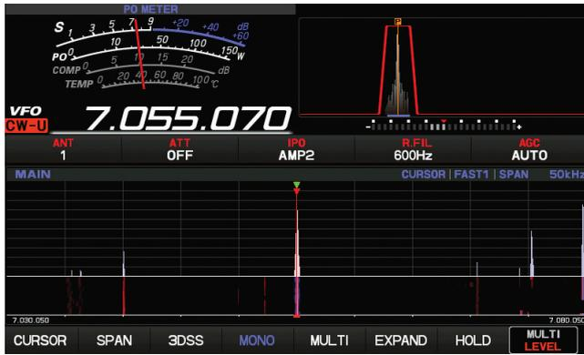
**Figure 1** — The Yaesu FTDX101D display showing a single waterfall view for 50 kHz of the 40-meter band centered at the frequency tuned by VFO A. The “filter function display” at the upper right shows the received passband with the received signal within. The spectrum span can be adjusted from a width of 1 kHz to 1 MHz in 10 steps.
