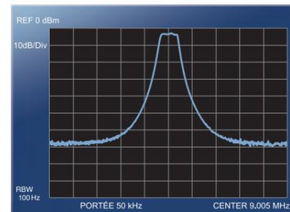
Filtre roofing 3 kHz (9 MHz, GAMME : 50 kHz)
