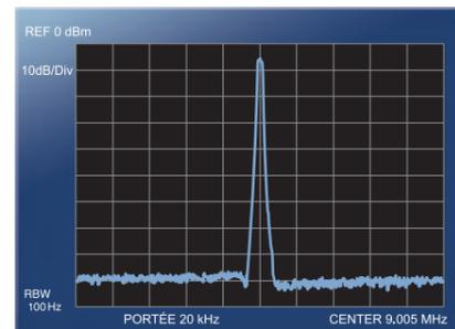
Filtre roofing 300 Hz (9 MHz, GAMME : 20 kHz)
