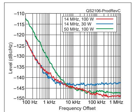
**Figure C** — The spectral display of the Yaesu FT<sub>DX</sub>10 transmitter output during phase-noise testing. Power output is 100 W on the 14 MHz band (red trace), 30 W on the 14 MHz band (blue trace), and 100 W on the 50 MHz band (green trace). The carrier, off the left edge of the plot, is not shown. This plot shows phase noise 100 Hz to 1 MHz from the carrier. The reference level is -110 dBc/Hz, and the vertical scale is 5 dB per division.
