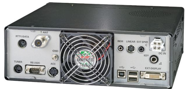
Figure 2 — The FTdx10 rear panel has connections for a variety of accessories. There is only one antenna jack, and no provision for a separate receive antenna. Note that the fan cycles on and off at slow speed in receive.
