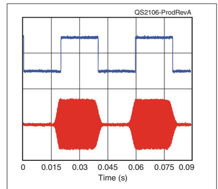
**Figure A** — The CW keying waveform for the Yaesu FT<sub>DX</sub>10, showing the first two dits in full-break-in (QSK) mode, using external keying and the default 6-millisecond rise time setting. Equivalent keying speed is 60 WPM. The upper trace is the actual key closure; the lower trace is the RF envelope. (Note that the first key closure starts at the left edge of the figure.) Horizontal divisions are 10 ms. The transceiver was being operated at 100 W output on the 14 MHz band.
