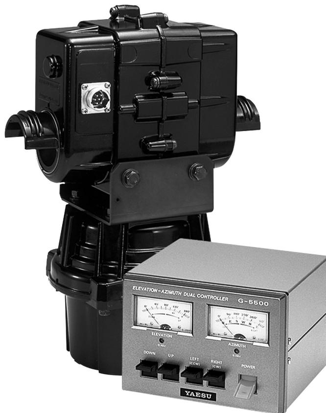
The Yaesu G-5500DC provide 450° azimuth and 180° elevation control of medium- and large-size unidirectional satellite antenna arrays under remote control from the station operating position. The rotators may be mounted together on a mast, or independently with the azimuth rotator inside a tower and the elevation rotator on the must.
