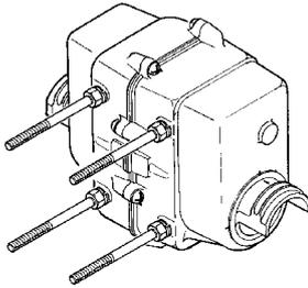
2. Slip an 8 mm flat washer over each installed stud bolt, and then the pipe clamps. Place another flat washer and then a spring washer over the end of each stud bolt, and start a nut on each to hold the hardware in place.
