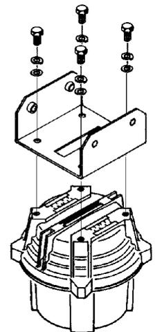
2. Insert the elevation rotator into the U-bracket, then fasten the elevation rotator using four M8x25 bolts, spring washers and flat washers.
