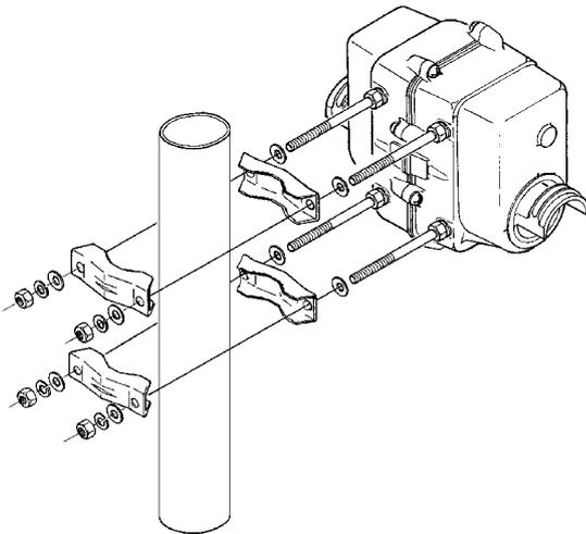
**Installing the boom in the Elevation Rotator.**
