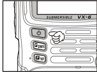
*1) If you don't hear the two "Beep" tones when the radio comes on, the Beeper may have been disabled via the Menu system. See page 21, which tells you how to reactivate the Beeper.*
