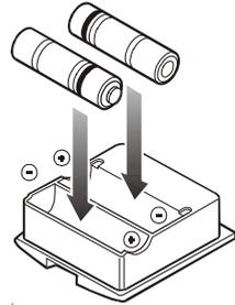
The **FBA-23** does not provide connections for charging, since Alkaline cells cannot be re-charged. Therefore, the **SAD-24**, **SDD-13**, or **E-DC-6** may safely be connected to the **EXT DC** jack when the **FBA-23** is installed.
