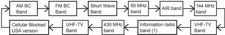
**Tip** Pressing  $\overline{\text{MW}}$  and then  $\overline{\text{SCOPE BAND DN (BAND)}}$  changes frequency bands shown above in the reverse order.
