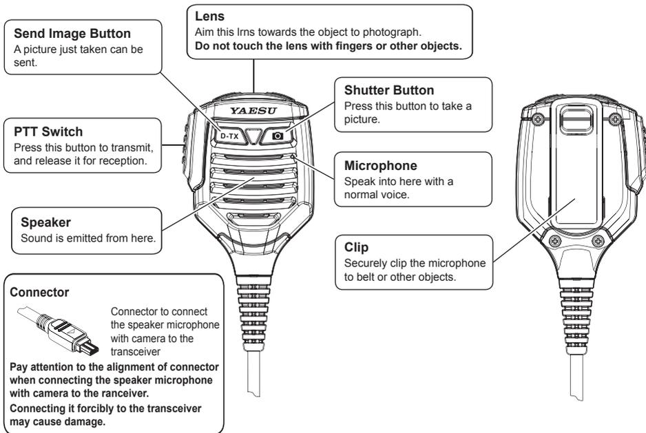
1 Connect the speaker microphone with camera (MH-85A11U) to the DATA terminal of the transceiver.
