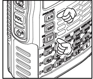
Each time <sup>MONO/DUAL</sup> (A/B) is pressed, the operating content displayed on the LCD screen is changed.
