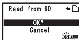
Blinks when reading is in progress
