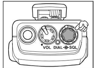
If you press the **[F/W]** key momentarily, then rotate the **DIAL**, frequency steps of 1 MHz will be selected. This feature is extremely useful for making rapid frequency excursions over the wide tuning range of the **FT-60R/E**.
