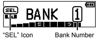
3. Press and hold the **F** key to copy the memory channel data into the Memory Bank. The blinking Bank Number stops blinking.
