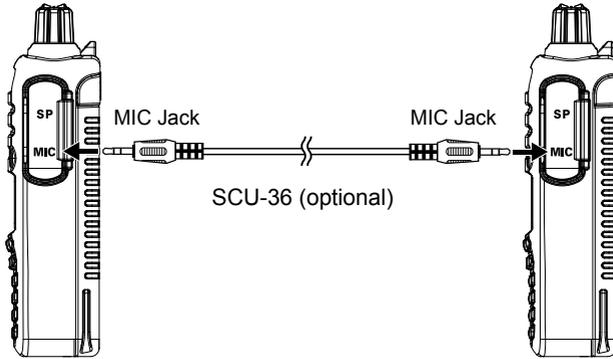
3. Press and hold the **MONI/T.CALL** key and the **PTT** switch simultaneously, while turning the transceiver ON.
