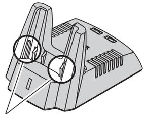
Align the slots of the battery pack with the guides in the nest of the **CD-30** Desktop Charger.
