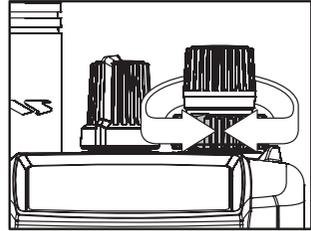
Adjust the **SQL** control just to the point where the noise is silenced and the LED is extinguished. If the **SQL** control is set further clockwise, sensitivity to weak signals will be reduced. Now, whenever a signal reaches the receiver that is strong enough to open the squelch, the indicator will glow green.
