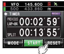
The lap time measured in the past will be displayed when **[RECALL]** is touched. When there are multiple lap times, touch **[▲]** or **[▼]** to switch between the lap times.
