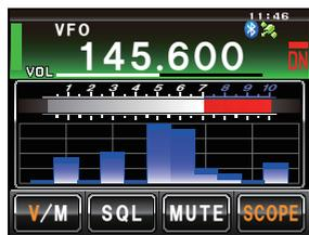
**Tip** The width of the band scope can be set to either “WIDE” or “NARROW” under **[DISPLAY]→[4 BAND SCOPE]** in the set-up menu.
