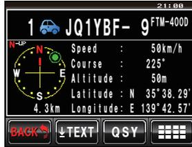
When using the APRS function, the call sign and symbol etc. of your own station need to be set (initial settings).
