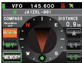
**COMPASS** Displays the compass settings. There are two settings, “Heading Up” where the direction of travel is on top, and “North Up” where North is always on top. Refer to “Change the Compass Settings” (P.94) for details.
