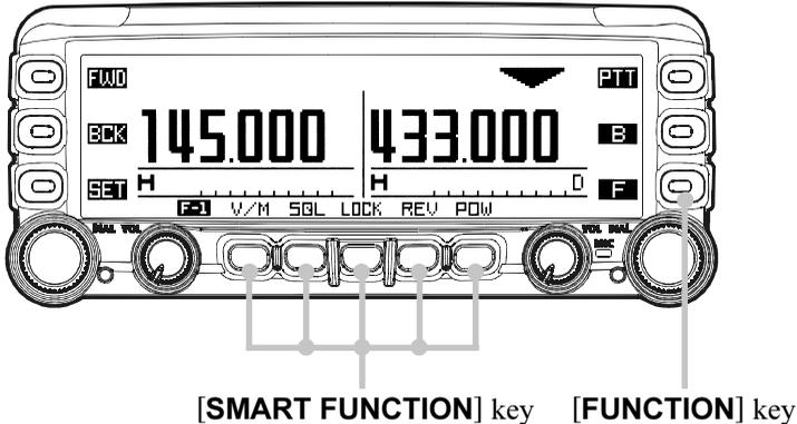
Pressing the [**F**] key repeatedly will change the function command of each [**SMART FUNCTION**] key as shown in the following tables. It is easy to recall and perform a desired operation. The current function of each key is shown in the display above the key button.
