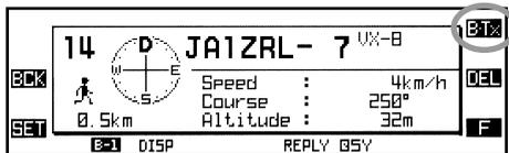
You may transmit your APRS beacon manually from the frequency display window. To do this, press the [F] key repeatedly, until the [SMART FUNCTION] key category changes to “F-3” mode, if necessary, then press the [B-TX] key.
