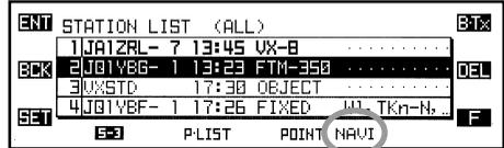
3. Press the [F] key repeatedly, until the [SMART FUNCTION] key's category changes to "S-3" mode, then press the [NAVI] key to open the "NAVI" page and initiate navigation. Drive your vehicle so that the "CAR" icon is pointing toward the "D" symbol in the Compass display.
