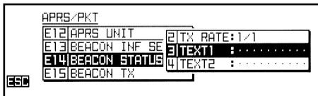
4. Rotate the *left side* **[DIAL]** knob to select the Status Text Register (“3: TEXT 1” through “7: TEXT 5”) you wish to store the text message to.
