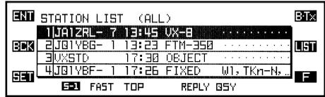
2. Rotate the *left side* [DIAL] knob to select the APRS station which you wish to navigate to.
