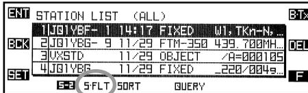
3. Press the *left side* [DIAL] knob, then rotate the *left side* [DIAL] knob to select the sort method.
