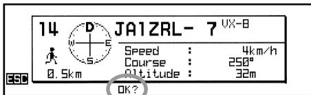
The **FTM-350** Series transceiver enables you to store up to 100 stations into the “Station” list.
