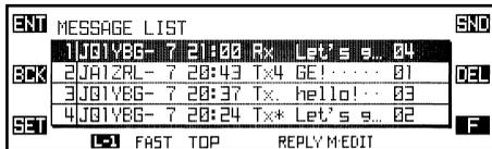
12. Each time the APRS message is transmitted repeatedly, the remaining number of transmissions of the message is shown on the display. If there is no acknowledgment packet (“ack”), even after the message transmits five times, the “.” (period) icon will appear on the “Message List” window, (Or, the “TXOut” notation will appear on the Message data window) instead of the remaining number of transmissions.
