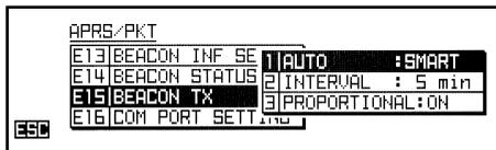
※: SmartBeaconing™ is an algorithm created by Tony Arnerich KD7TA and Steve Bragg KA9MVA of HamHUD for adjusting the transmit rate using the speed and heading changes of the vehicle.
