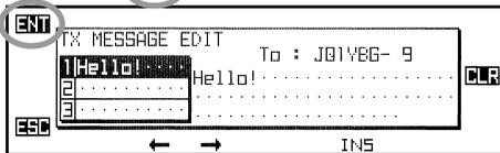
10. When the message entry is complete, press the [M•TX] key to transmit the message and return to the normal operation display. The transmitted message is stored into the “Message List”.
