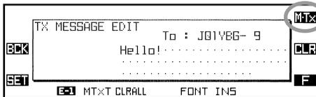
11. The APRS message is transmitted repeatedly, up to five times, once each minute until an acknowledgment packet (“ack”) is received. If an acknowledgment packet (“ack”) is received, the beeper will sound and the “\*” icon will appear on the display.
